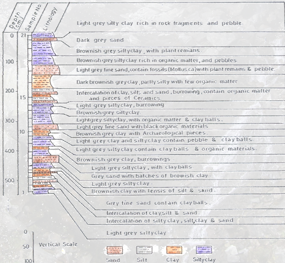
Fig.2. Stratigraphic section of Euphrates Flood-Plain (Barwanah area).
