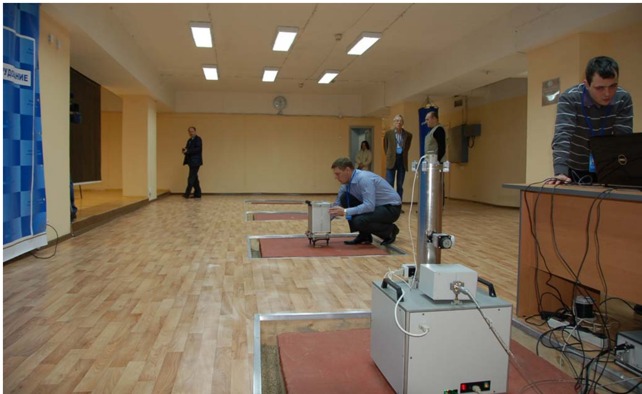
Fig. 5 Comparison of absolute gravity meters at the site of East Siberian Division of the Federal Service of Registration, Cadastre and Cartography
