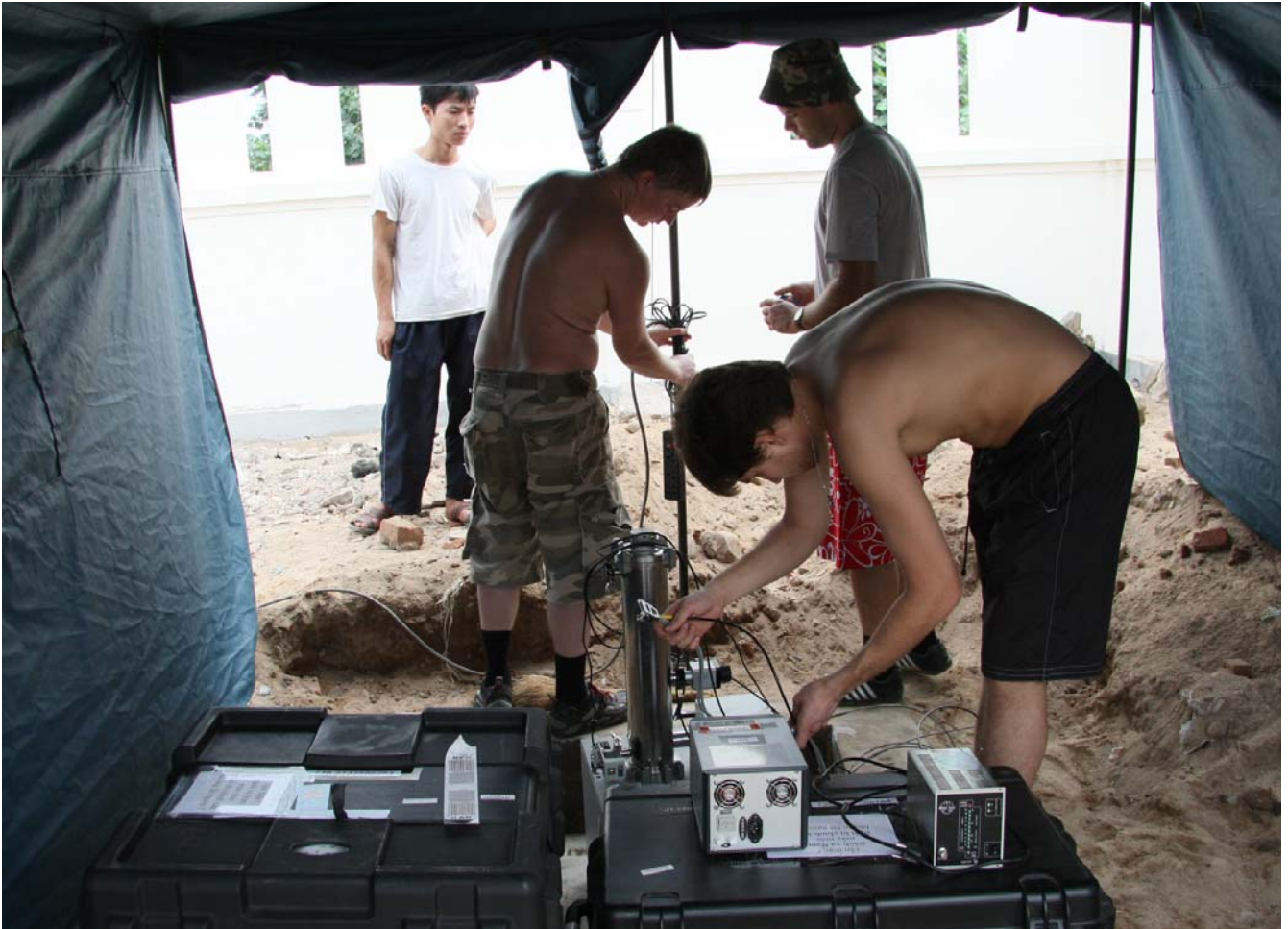
Fig.7 Absolute gravity measurement at a field gravimetric point.
